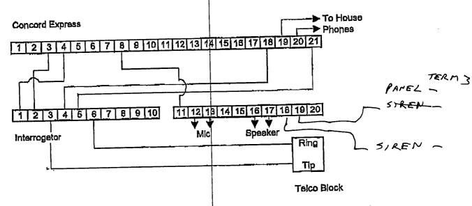
The Interrogator trip on the Express panel was designed to make it an easy installation for the tech. The Interrogator should work, out of the box, just the same as the Commander 2000. Using the trip 018, the panel sends a 2-way signal to the Central Station. It will only work with instant activation. The Trip form the panel should be configured on output 2 as 01800.
